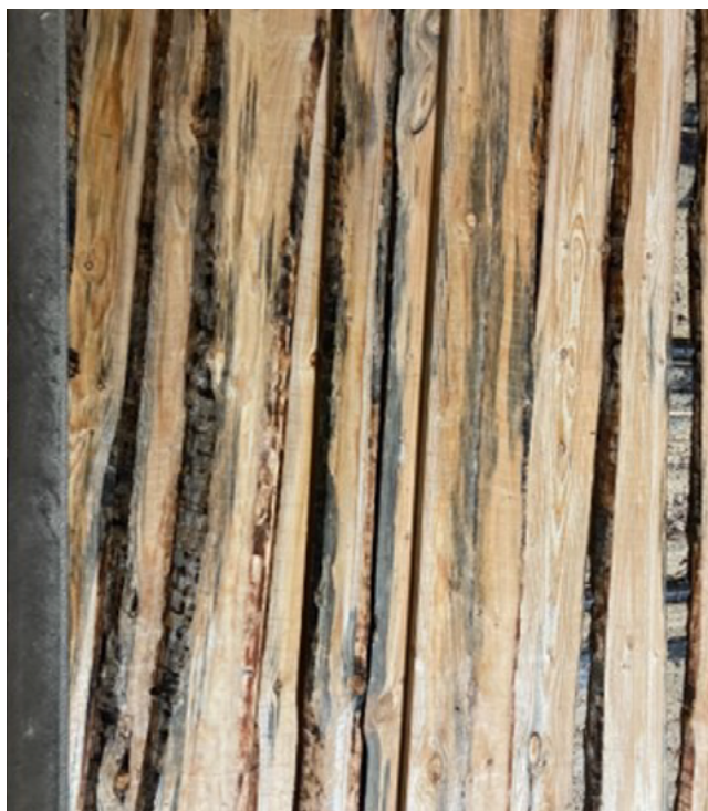
Photo 6-5: Photos of trial logs prior to and after breaking down showing level of blue stain July 2022. Source: FCNSW
