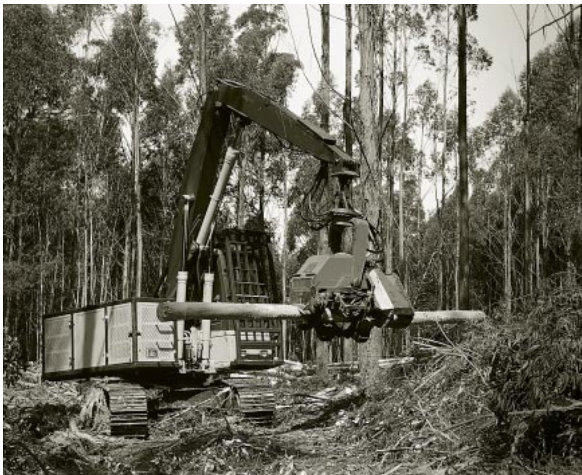
A single grip harvester in operation in native forest.
