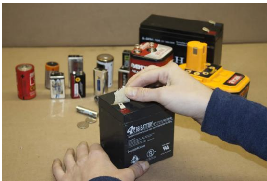
Figure 1: Using masking tape to seal the positive terminal on a sealed lead acid battery
